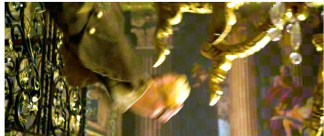
(c) Checkerboard visualization of color mismatch between the original left view and the left view reconstructed from the right view.
